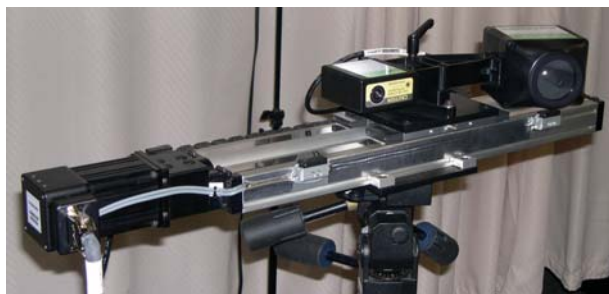
Fig. 1. The ShapeGrabber® PLM300 Laser Scanner System features a linear motion range of 300 mm and accuracy of 0.05 mm. The scan head, SG-1000, has a depth field of 250-900 mm and a depth accuracy of 5.0 \mu\text{m} at the farthest point.
