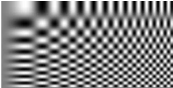
Fig. 3. A synthetic test pattern deployed by sine-wave gratings, which are optimally tuned to the HVS. The test images are perturbed by Poisson noise for the assessment.
