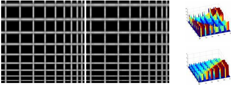
Fig. 4. (left, middle) Intensity corrected images using the mean-weight filtering with the kernel size of 33 (left) and 47 (middle) respectively. (right) Intensity correction maps (pseudo colored) where upper and lower map corresponds to the (left) and (middle) image respectively.
